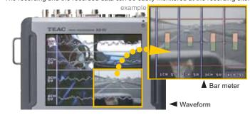
4 channels per screen or full screen viewing ( selected channels ) Waveform / Bar meter : 4 selectable waveform or bar meter ( overlav )
